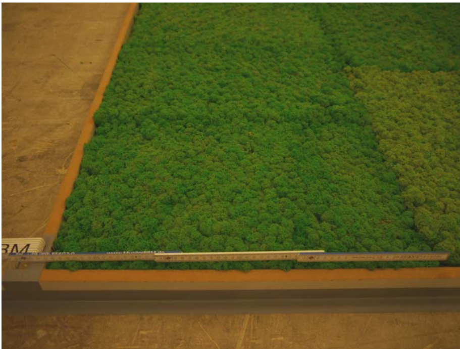
Figure B.2. Enclosing frame sealed with adhesive tape.
